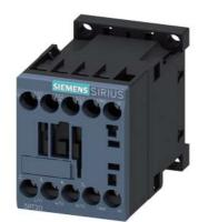
Power contactor, AC-3 9 A, 4 kW / 400 V 1 NO, 24 V AC, 50 / 60 Hz 3-pole, Size S00 screw terminal
