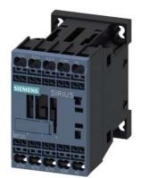
Power contactor, AC-3 7 A, 3 kW / 400 V 1 NC, 230 V AC, 50/60 Hz 3-pole, size S00 Spring-type terminal
