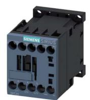
Power contactor, AC-3 7 A, 3 kW / 400 V 1 NO, 110 V AC, 50 / 60 Hz 3-pole, Size S00 screw terminal
