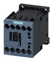
Power contactor, AC-3 7 A, 3 kW / 400 V 1 NC, 24 V AC, 50 / 60 Hz 3-pole, Size S00 screw terminal
