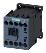
Power contactor, AC-3 7 A, 3 kW / 400 V 1 NO, 24 V AC, 50 / 60 Hz 3-pole, Size S00 screw terminal
