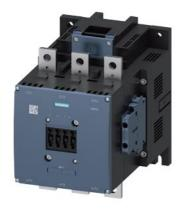
Power contactor, AC-3 500 A, 250 kW / 400 V AC (50-60 Hz) / DC 220-240 V UC Auxiliary contacts 2 NO + 2 NC 3-pole, size S12 Busbar connections Operating mechanism: conventional screw terminals
