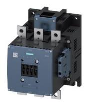
Power contactor, AC-3 265 A, 132 kW / 400 V AC (50-60 Hz) / DC operation 110-127 V UC Auxiliary contacts 2 NO + 2 NC 3-pole, Size S10 Busbar connections Drive: conventional screw terminal
