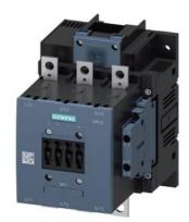
Power contactor, AC-3 150 A, 75 kW / 400 V AC (50-60 Hz) / DC operation 110-127 V UC Auxiliary contacts 2 NO + 2 NC 3-pole, Size S6 Busbar connections Drive: conventional screw terminal
