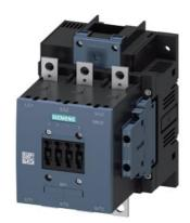
Power contactor, AC-3 150 A, 75 kW / 400 V AC (50-60 Hz) / DC operation 23-26 V UC Auxiliary contacts 2 NO + 2 NC 3-pole, Size S6 Busbar connections Drive: conventional
