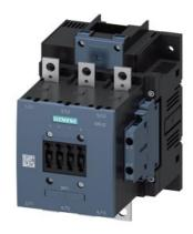
Power contactor, AC-3 115 A, 55 kW / 400 V AC (50-60 Hz) / DC operation 110-127 V UC Auxiliary contacts 2 NO + 2 NC 3-pole, Size S6 Busbar connections Drive: conventional screw terminal
