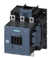
Power contactor, AC-3 115 A, 55 kW / 400 V AC (50-60 Hz) / DC operation 23-26 V UC Auxiliary contacts 2 NO + 2 NC 3-pole, Size S6 Busbar connections Drive: conventional screw terminal
