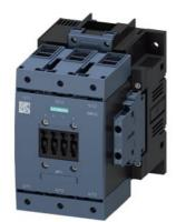
Power contactor, AC-3 115 A, 55 kW / 400 V AC (50-60 Hz) / DC operation 110-127 V UC Auxiliary contacts 2 NO + 2 NC 3-pole, Size S6 with box terminals Drive: conventional screw terminal
