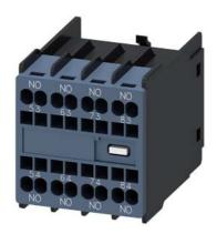
Auxiliary switch on the front, 4 NO Current path 1 NO, 1 NO, 1 NO, 1 NO for contactor relays Size S00 spring-type terminal 53/54, 63/64, 73/74, 83/84 Physically coded; only with contactor relays 3RH2140\* and 3RH2440\* can be combined (according to EN 50011)
