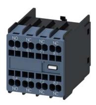
Auxiliary switch on the front, 1 NO + 3 NC Current path 1 NO, 1 NC, 1 NC, 1 NC for contactor relays Size S00 spring-type terminal 51/52, 61/62, 71/72, 81/82 Physically coded; only with contactor relays 3RH2140\* and 3RH2440\* can be combined (according to EN 50011)
