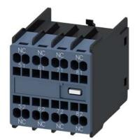
Auxiliary switch on the front, 4 NC Current path 1 NC, 1 NC, 1 NC, 1 NC for contactor relays Size S00 spring-type terminal 51/52, 61/62, 71/72, 81/82 Physically coded; only with contactor relays 3RH2140\* and 3RH2440\* can be combined (according to EN 50011)
