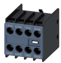
Auxiliary switch on the front, 4 NO Current path 1 NO, 1 NO, 1 NO, 1 NO for contactor relays Size S00 screw terminal 53/54, 63/64, 73/74, 83/84 for 3RH2140/3RH2440 acc. to EN 50011 Physically coded; only with contactor relays 3RH2140\* and 3RH2440\* can be combined (according to EN 50011)
