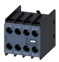
Auxiliary switch on the front, 4 NC Current path 1 NC, 1 NC, 1 NC, 1 NC for contactor relays Size S00 screw terminal 51/52, 61/62, 71/72, 81/82 Physically coded; only with contactor relays 3RH2140\* and 3RH2440\* can be combined (according to EN 50011)
