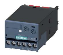
Electronic timing relay OFF delay With control signal and semiconductor output 90-240 V AC/DC Time range 0.05...100 s Can be snapped on at the front For contactors 3RT2, S2, S3 and 3RH2 S00 contactor relays Screw terminal
