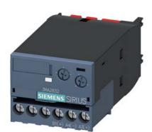
Electronic timing relay OFF delay With control signal and semiconductor output 24-90 V AC/DC Time range 0.05...100 s Can be snapped on at the front For contactors 3RT2, S2, S3 and 3RH2 S00 contactor relays Screw terminal
