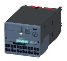
Electronic timing relay ON delay With semiconductor output 90-240 V AC/DC Time range 0.05...100 s Can be snapped on at the front For contactors 3RT2, S2, S3 and 3RH2 S00 contactor relays Spring-type
