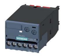
Electronic timing relay ON delay With semiconductor output 90-240 V AC/DC Time range 0.05...100 s Can be snapped on at the front For contactors 3RT2, S2, S3 and 3RH2 S00 contactor relays Screw terminal
