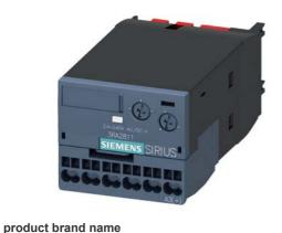
Electronic timing relay ON delay with semiconductor output 24-240 V AC/DC Time range 0.05...100 s can be snapped on at the front for contactors 3RT2 S00/S0 and auxiliary contactor 3RH2 S00 Spring-type terminal Varistor for attenuation of the contactor coils integrated
