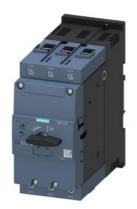
Circuit breaker size S3 for motor protection, Class 20 A-release 80...100 A N-release 1300 A screw terminal Increased switching capacity 100 kA  $\,$
