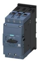
Circuit breaker size S3 for motor protection, CLASS 10 A-release 57...75 A N-release 975 A screw terminal Increased switching capacity 100 kA
