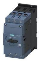
Circuit breaker size S3 for motor protection, Class 20 A-release 28...40 A N-release 520 A screw terminal Increased switching capacity 100 kA  $\,$
