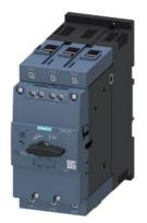
Circuit breaker size S3 for motor protection, CLASS 10 A-release 65...84 A N-release 1170 A screw terminal Standard switching capacity with transverse auxiliary switches 1 NO+1 NC  $\,$
