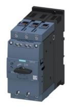
Circuit breaker size S3 for motor protection, CLASS 10 A-release 80...100 A N-release 1300 A screw terminal Standard switching capacity with transverse auxiliary switches 1 NO+1 NC
