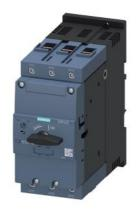
Circuit breaker size S3 for motor protection, CLASS 10 A-release 80...100 A N-release 1300 A screw terminal Standard switching capacity
