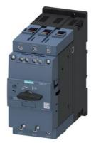
Circuit breaker size S3 for motor protection, CLASS 10 A-release 28...40 A N-release 520 A screw terminal Standard switching capacity with transverse auxiliary switches 1 NO+1 NC  $\,$
