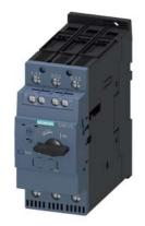
Circuit breaker size S2 for motor protection, CLASS 10 A-release 49...59 A N-release 845 A screw terminal increased switching capacity with transverse auxiliary switches 1 NO+1 NC
