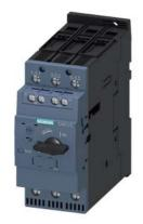
Circuit breaker size S2 for motor protection, CLASS 10 A-release 42...52 A N-release 741 A screw terminal increased switching capacity with transverse auxiliary switches 1 NO+1 NC
