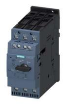
Circuit breaker size S2 for motor protection, CLASS 10 A-release 32...40 A N-release 585 A screw terminal increased switching capacity with transverse auxiliary switches 1 NO+1 NC
