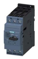
Circuit breaker size S2 for motor protection, CLASS 10 A-release 62...73 A N-release 949 A screw terminal increased switching capacity
