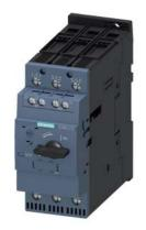
Circuit breaker size S2 for motor protection, CLASS 10 A-release 54...65 A N-release 845 A screw terminal increased switching capacity with transverse auxiliary switches 1 NO+1 NC
