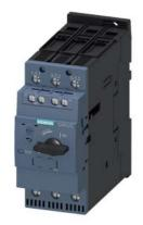
Circuit breaker size S2 for motor protection, CLASS 10 A-release 22...32 A N-release 416 A screw terminal increased switching capacity with transverse auxiliary switches 1 NO+1 NC
