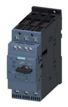
Circuit breaker size S2 for motor protection, CLASS 10 A-release 49...59 A N-release 845 A screw terminal Standard switching capacity with transverse auxiliary switches 1 NO+1 NC
