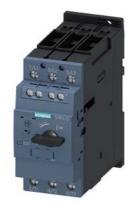
Circuit breaker size S2 for motor protection class 20 A-release 35...45 A N-release 650 A screw terminal Standard switching capacity with transverse auxiliary switch 1 NO+1 NC
