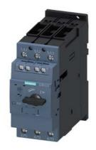
Circuit breaker size S2 for motor protection, CLASS 10 A-release 12...17 A N-release 260 A screw terminal Standard switching capacity with transverse auxiliary switches 1 NO+1 NC
