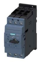
Circuit breaker size S2 for motor protection, Class 20 A-release 9.5...14 A N-release 208 A screw terminal Standard switching capacity
