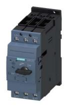
Circuit breaker size S2 for motor protection, CLASS 10 A-release 9.5...14 A N-release 208 A screw terminal Standard switching capacity
