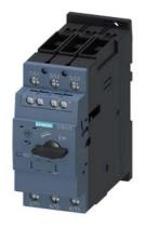
Circuit breaker size S2 for motor protection class 20 A-release 28...36 A N-release 520 A screw terminal Standard switching capacity with transverse auxiliary switch 1 NO+1 NC
