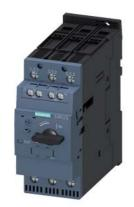
Circuit breaker size S2 for motor protection class 20 A-release 54...65 A N-release 845 A screw terminal Standard switching capacity with transverse auxiliary switches 1 NO+1 NC
