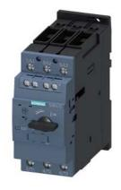
Circuit breaker size S2 for motor protection, Class 20 A-release 22...32 A N-release 416 A screw terminal Standard switching capacity with transverse auxiliary switches 1 NO+1 NC
