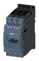
Circuit breaker size S2 for motor protection, CLASS 10 A-release 18...25 A N-release 325 A Screw terminal Standard switching capacity with transverse auxiliary switches 1 NO+1 NC
