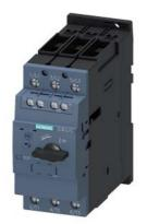
Circuit breaker size S2 for motor protection class 20 A-release 14...20 A N-release 260 A screw terminal Standard switching capacity with transverse auxiliary switch 1 NO+1 NC
