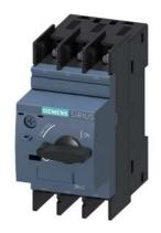
Circuit breaker size S0 for motor protection, CLASS 10 A-release 18...25 A N-release 325 A ring cable lug connection Standard switching capacity
