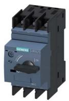
Circuit breaker size S0 for motor protection, CLASS 10 A-release 16...22 A N-release 286 A ring cable lug connection Standard switching capacity
