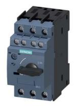
Circuit breaker size S0 for motor protection, CLASS 10 A-release 16...22 A N-release 286 A screw terminal Standard switching capacity with transverse auxiliary switches 1 NO+1 NC
