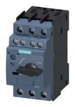
Circuit breaker size S0 for motor protection, CLASS 10 A-release 13...20 A N-release 260 A screw terminal Standard switching capacity with transverse auxiliary switches 1 NO+1 NC
