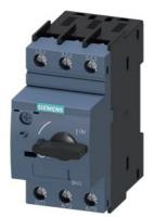
Circuit breaker size S0 for motor protection, CLASS 10 A-release 5.5...8 A N-release 104 A screw terminal Standard switching capacity
